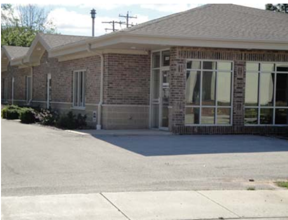
This building is relatively close to the sidewalk, but people have to travel through the parking lot to reach the door from the sidewalk.
